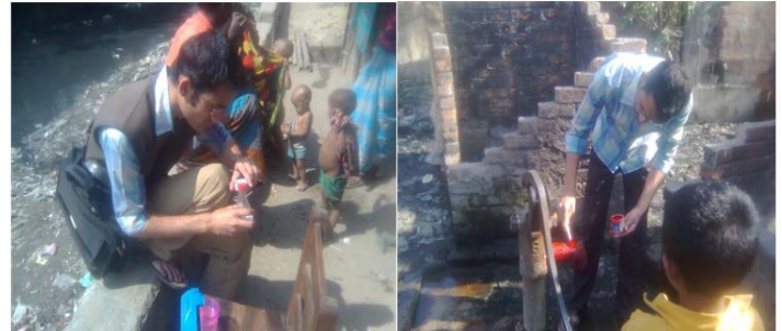
Fig. 3. Testing of samples on the field and painting of arsenic detected tube wells with red color.
